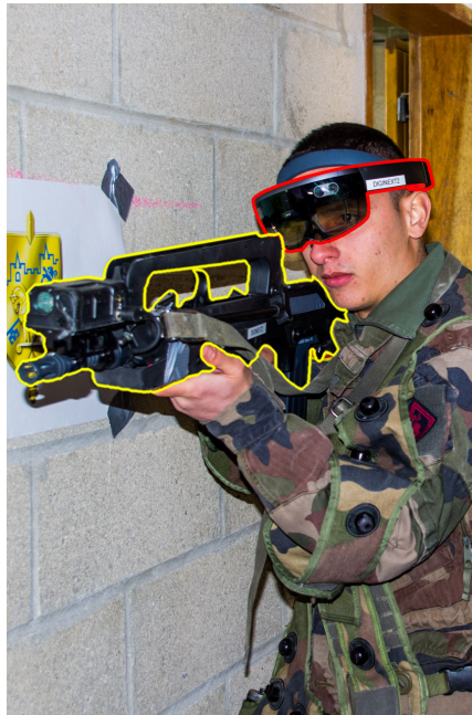
Figure 6 : The SIMBA prototype, made of HoloLens glasses (outlined in red), and the FAMAS replica equipped with the laser emitter (outlined in yellow)
